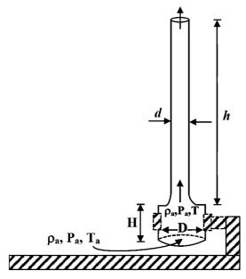
16. Considering the air flow to be streamline, the steady mass flow rate of air exiting the chimney is \_\_\_\_\_ gm s<sup>-1</sup>.
